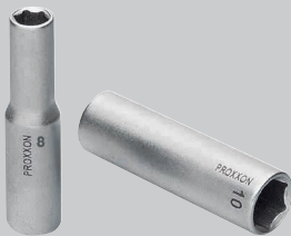
3/8" deep sockets for protruding bolts. Made of CrV steel. Total length 46mm.
